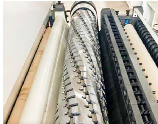
Planer carbide knives spiral along the planer head
