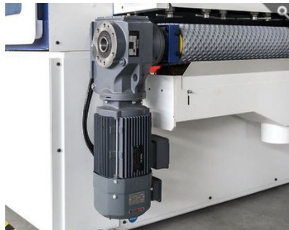
Helical bevel gear integrated inverter motor
